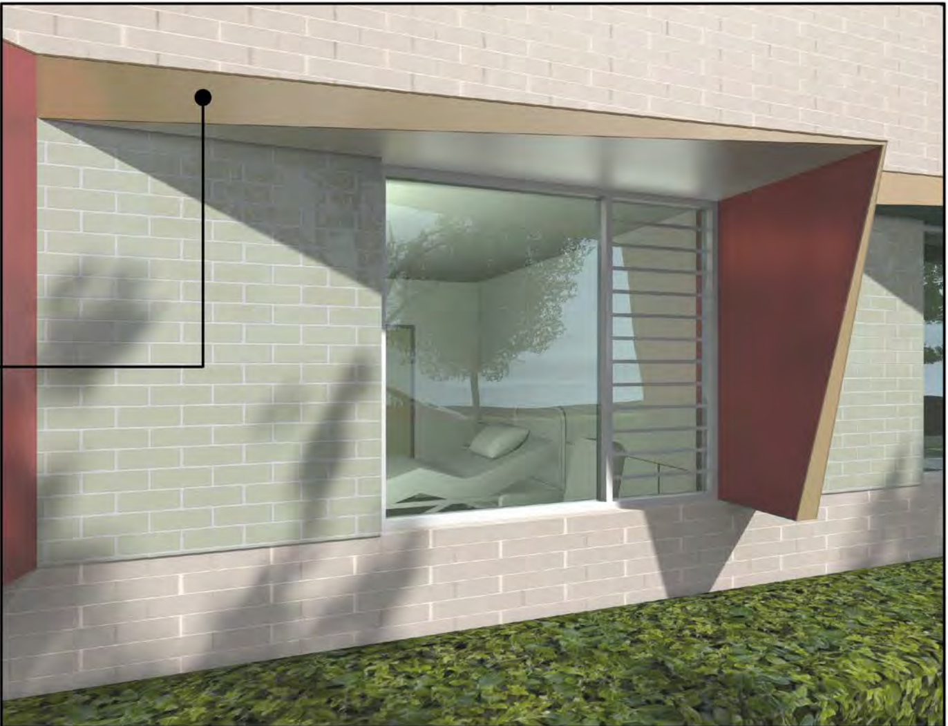
Coloured aluminium sun-hood panels
